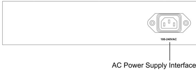
**Figure 3-2. Attaching AC Power Cable to Device**
